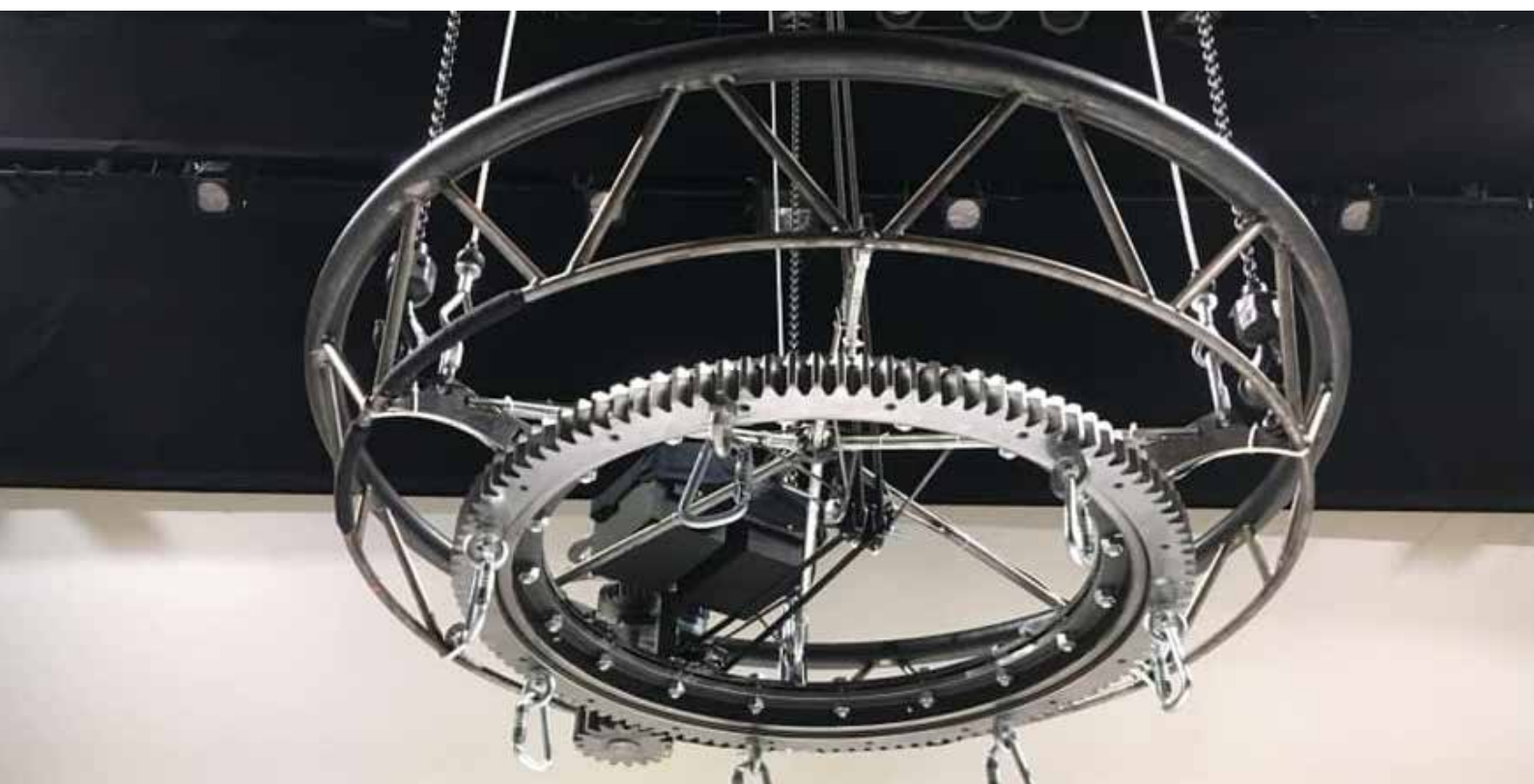
Motorised circle truss for flying trapeze designed by Eric Abadie, Aérée
